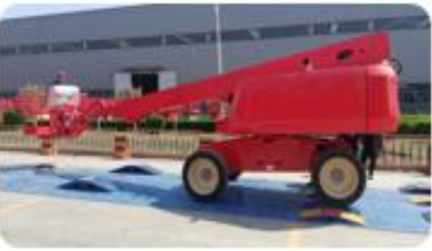
Angle alarm test
